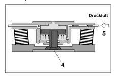
In the FM's locked condition, the tool flange and the robot flange form a rigid unit.
